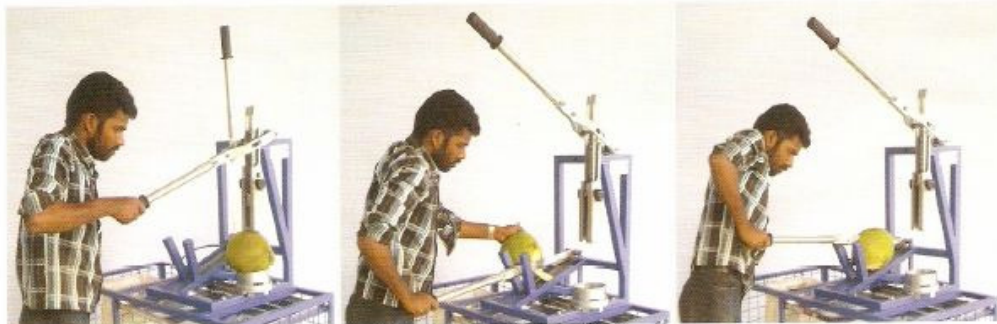
Operating the punch cum splitter
