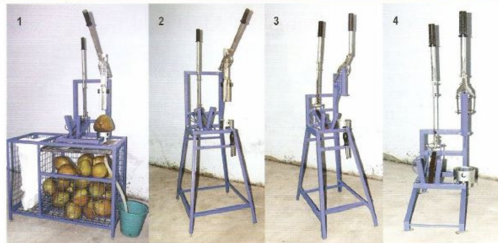
1. Punch cum splitter, 2. Economy punch cum splitter, 3. Handy punch cum splitter, 4. Table top punch cum splitter
